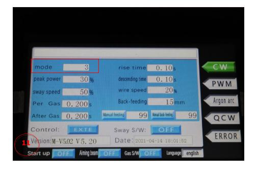
8) The machine screen come with 0 to 31 mode parameter. Each mode corresponds to different setting parameters, and the welding parameters of the corresponding material can be saved.
