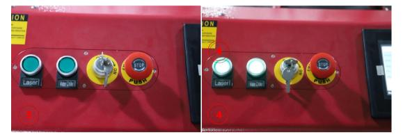
2) Turn on Emergency, key switch to On position, Laser, Water chiller button.
