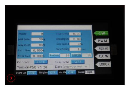
4) CW mode: Peak power rate adjust 5 to 100% range, rise time 0.0 s, descending time 0.20s,sway speed 12 to 100% range, Per gas 0.3 to 0.5 s, After gas 0.3 s, Wire speed 1 to 100%, Back-feeding 1 to 99mm range, manual feeding 0 to 99mm, manual back-feeding 0 to 99mm.
