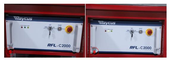
**3)** Turn on Emergency, key switch to REM position, When green light is On, laser source working. **Don't press start button on the laser source.**
