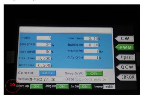
7) If you want to weld aluminum material, you have to adjust mode to PWM After change modulation frequency 1 to 15000Hz, normally use 10000Hz. Duty cycle adjust 20% to 100%,normally use 85% duty cycle for weld aluminum
