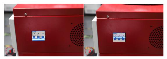
1) After connected well power supply of the machine. Turn on airswitch button like 2 picture.
